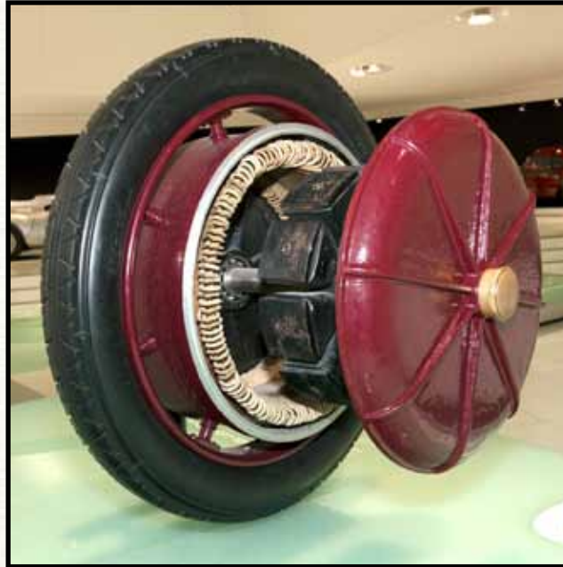
Lohner-Porsche electric wheel hub motor from 1900, now in the Porsche Museum in Germany. Photo by Morio and used under the Creative Commons Attribution-Share Alike 3.0 Unported license.
